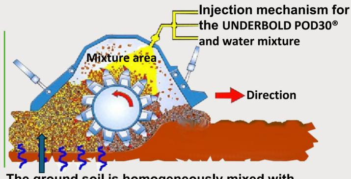
The ground soil is homogeneously mixed with the UNDERBOLD POD30®
